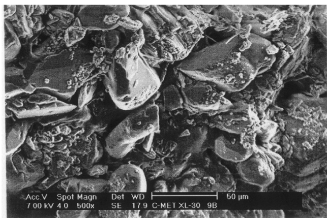
a) SEM micrograph of control formulation, 500x
