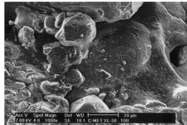
d) SEM micrograph of control with 5% NTO, 1000x
